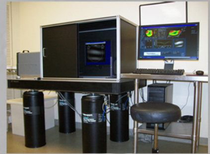
Phase Measuring Interferometer Flatness/Wedge/TWF
