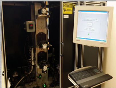
Three Stage Ellipsometer Polarization / Retardance
